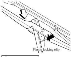
To prevent damage to the windshield let the wiper arm down easily, don't let it slap down on the windshield. 2. Hold the end of the rubber and pull until the tabs are free of the metal support.
